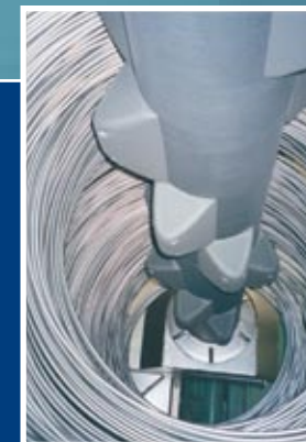
Mandrel ensures full exposure & complete cleaning
