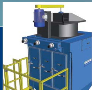
Roof mounted fans offer the ability to discharge air in any direction, as the base plate has a symmetrical bolt pattern that allows it to be rotated every 90 degrees.
