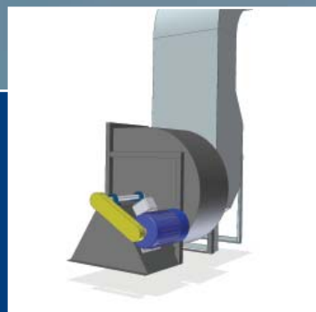
Floor mounted fans allow quick and easy maintenance access as well as eliminating any dynamic loads on the collector with large fans. All fans over 30 HP will be mounted on the floor.
