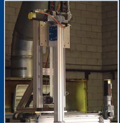
Roof (external) mounted Multi-axis Nozzle Carriage
