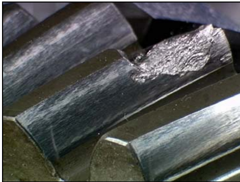
Figure 1: Fatigue Failure of a Gear Tooth
