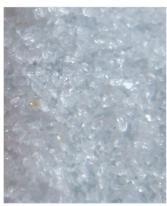
Wheelabrator Plus glass beads and glass grit are manufactured under strict quality control criteria. Glass Beads clean and remove surface deposits with a peening action leaving a lustrous surface finish. They are ideal for use on both ferrous and non ferrous surfaces and for use in both wet and dry blast machines. All Wheelabrator Plus glass products contain no free silica.
